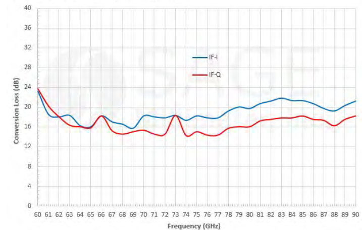
Typical Conversion Loss vs. Frequency
